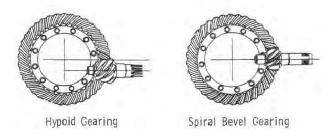
Before Packard, the standard of the industry was the spiral bevel gearset, as shown above. This ring-and-pinion configuration is nearly ancient in origin and relatively simple to produce, but it does have some drawbacks, including classic gear whine and limited tooth contact area. The centerline of the pinon (driving) gear is directly on the centerline of the ring (driven) gear.
